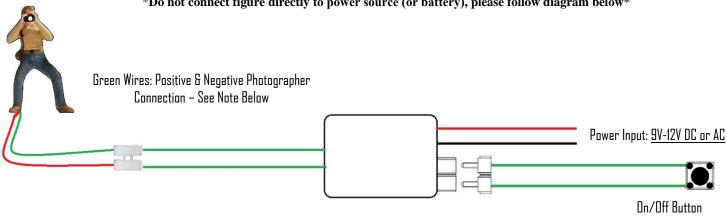
Note: If the flash doesn't light up on the first try, please flip the green wires and test again. No worries, there will be no damage to the flash if the polarity is reversed.
